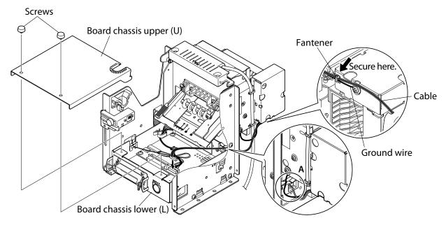
(4) Fit the board chassis upper (U) back onto the board chassis lower (L), and fasten in place with the two screws.
